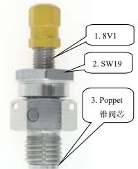
"2.SW19" by anticlockwise direction by spanner slowly until the pressure gauge signals. When the pressure reading is not go up, then stop turn the wheel and the pressure reading is the charging pressure of the accumulator.
